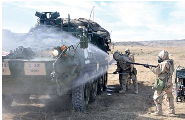
Figure 20: Land vehicle decontamination.
